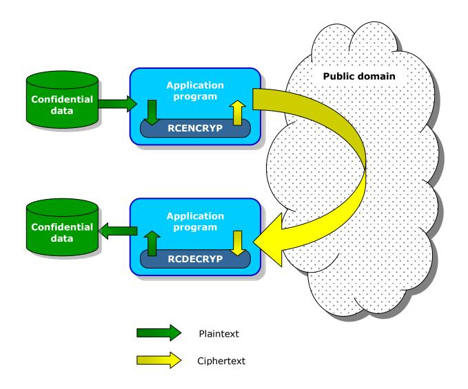
The Redvers Encryption Module runs the standard AES cipher, which means it can generate ciphertext for decryption by other AES ciphers and decrypt ciphertext, generated by other AES ciphers.
